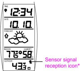
\* When the signal is successfully received by the Weather Station, the icon will be switched on. (If not successful, the icon will not be shown in LCD) So the user can easily see whether the last reception was successful (icon on) or not (icon off). On the other hand, the short blinking of the icon shows that a reception is being done now.
