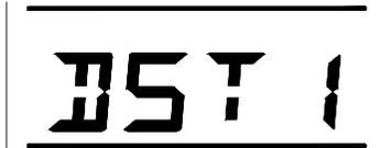
5. Press and release the *IN* button to select DST on or off.
